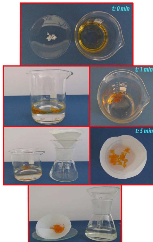
Figure 10. Process of separation of toluene (dyed with methyl red) from water surfaces. [Color figure can be viewed at wileyonlinelibrary.com.]
